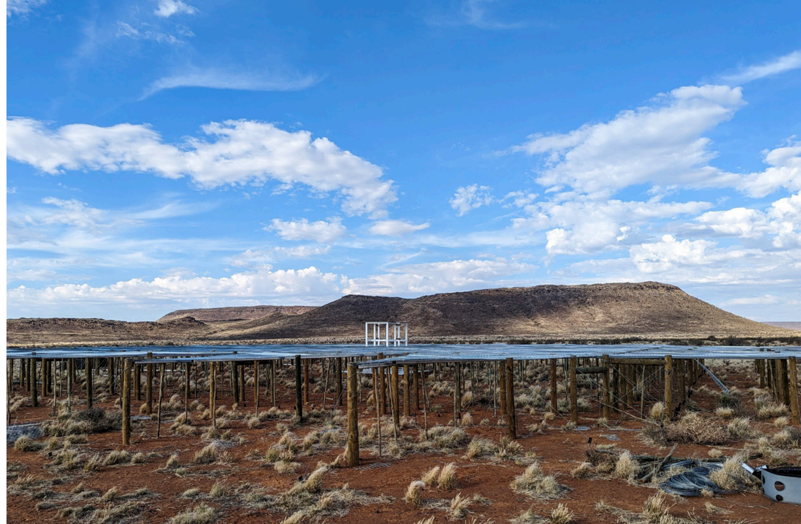
Fig.4 . REACH dipole antenna at the Karoo radio reserve, South Africa, a site ideally suited for radio astronomy and future location of the SKA-MID telescope. The antenna is placed over a 20x20 m elevated metallic mesh in order to shield the antenna from soil emission. Credit: Christian Kirkham.
