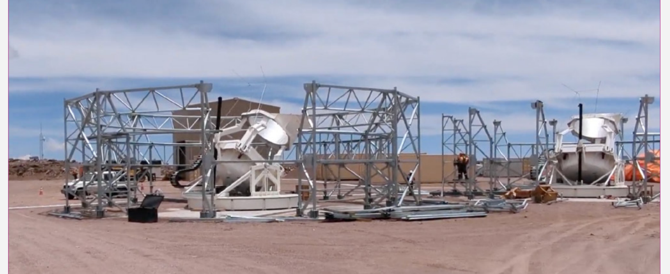
Fig. 1: Two of the three SATs, and their associated ground screens, on site in Chile. SO:UK will add a further two SATs and Japanese colleagues will provide a further one, totalling six.
