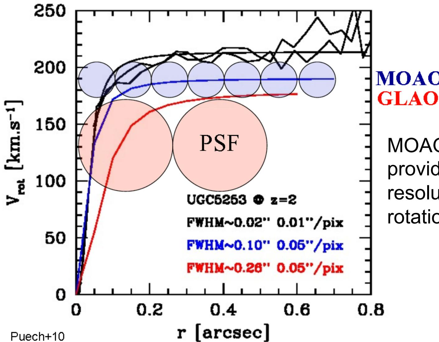
MOAO is required to provide at least 5 to 7 resolution elements per rotation curve side
