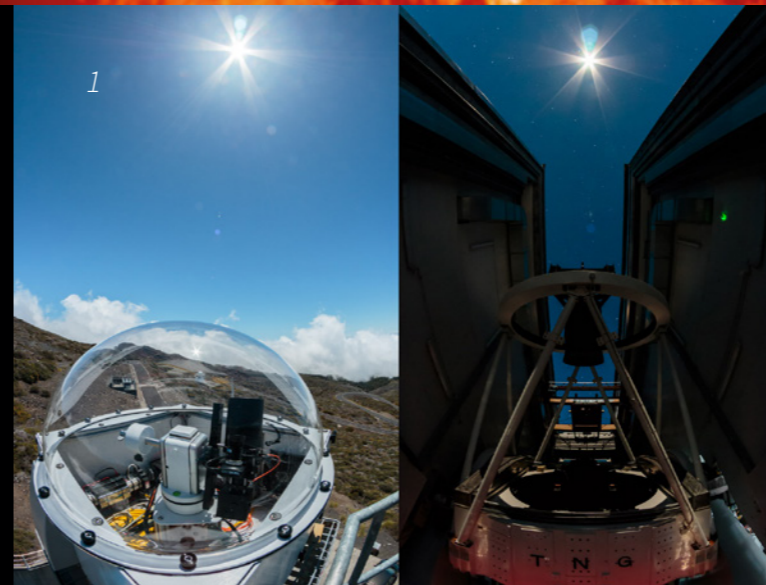
Fig 1. The small Solar Telescope (left) and the Telescopio Nazionale Galileo (right) both feeding into HARPS-N.
